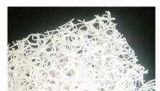
High strength polyethylene fiber "Tsunooga"
