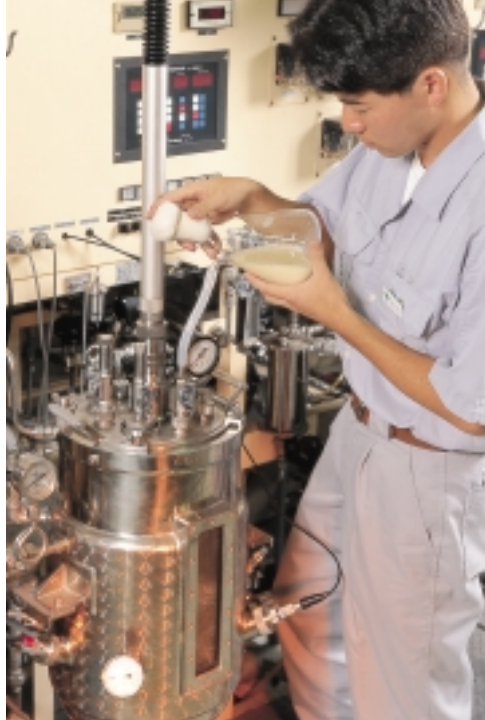
A 30-liter fermenter for cultivating microorganisms
