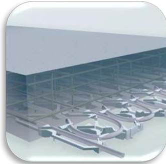
Thermally active building structures (TABS)
