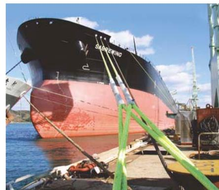
Mooring cable made of ultrahigh-strength polyethylene fiber “Dyneema”
