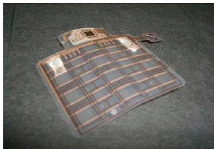
Heat curing type polyimide solder resist ink
