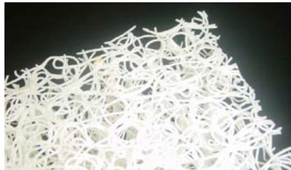
High strength polyethylene fiber "Tsunoooga"
