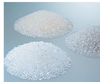
Polyester resins— "TOYOBO GS Catalyst" (front), antimony-based catalyst (right), and titan-based catalyst (back)
