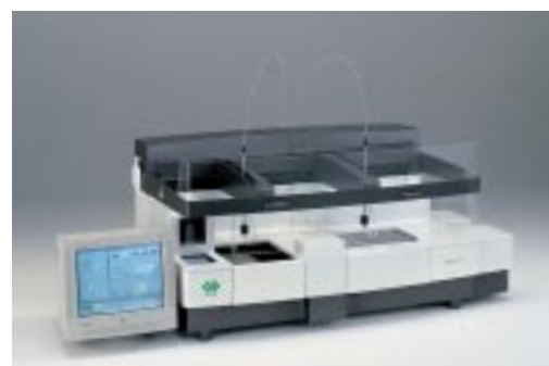
Allegro Lite, a fully automated immunochemiluminescent system
